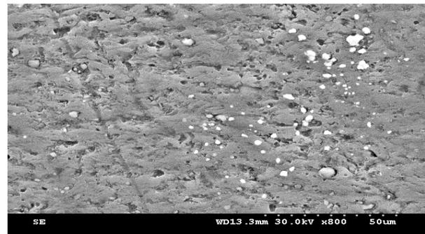
Fig. 5: SEM image of Al / Nano SiCp composite
