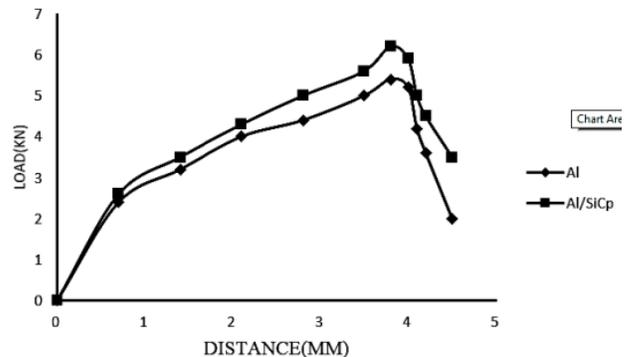
**Fig. 8: Comparison of compressive strength for Al and Al/Sic**
