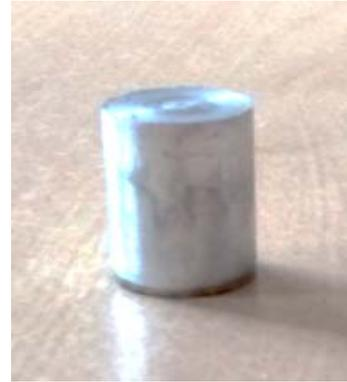
Fig. 3: Compacted Al/Nano SiCp Composite specimen
