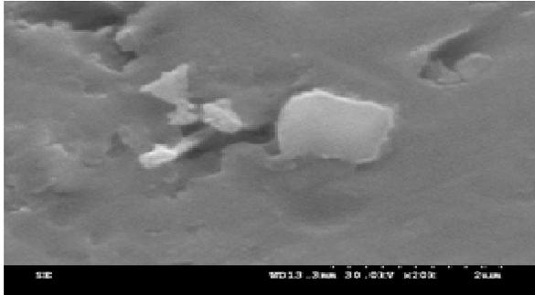
**Fig. 6: SEM image shows the presence of Nano SiC particle in the matrix**
