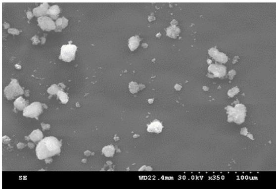
Fig. 1: SEM image of Nano SiCp
