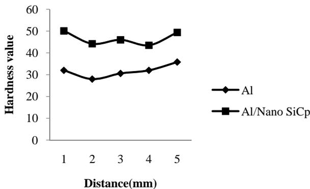
**Fig. 7: Comparison of Hardness for Al and Al/Sic**
